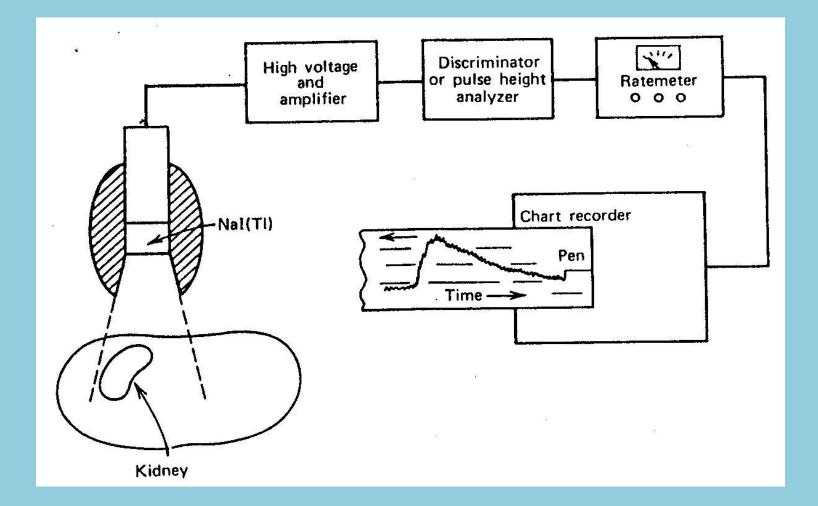
Kidney function is also often studied with scintillation detectors. About 7MBq  $(\sim 200 \mu ci)$  of <sup>131</sup>I labeled hipuric acid is injected into the bloodstream, and a sit is removed from the blood by the kidneys the radioactivity of each kidney is monitored and record the change in the radioactivity with time.
