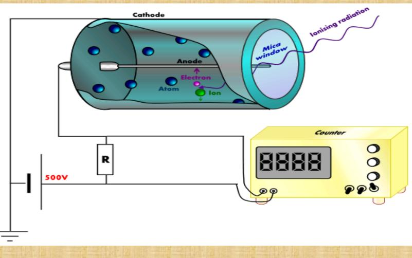
**Geiger tube consists of a wire anode** surrounding by a mental cathode, the space between them being filled with a mixture of gases (often argon or neon with a little bromine or chlorine) at low pressure. There is usually a small glass bead on end of the wire anode to prevent discharge from a point.
