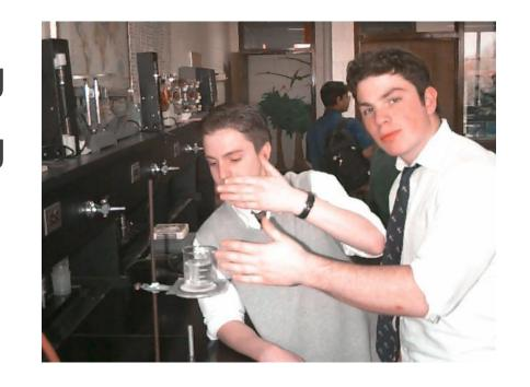
Use a rubber suction bulb , pump or other device to fill a pipette
