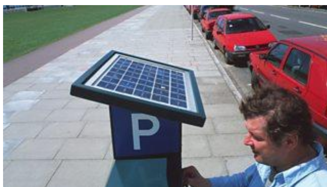
A solar panel on top of a parking ticket machine
